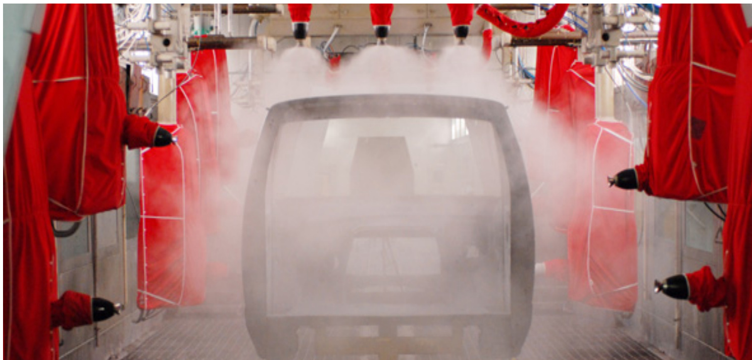
Paint is applied to an E-Series vehicle using a multicoat process at the Ford Ohio Assembly Plant.
